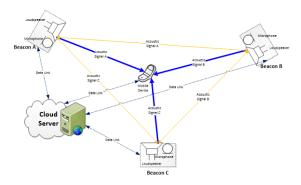
Figure 1: proposed Acoustic Positioning System Configuration
