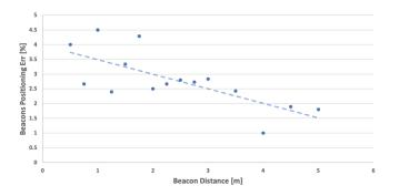
Figure 9: Beacons positioning error
