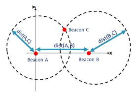
Figure 4: Beacons Positioning through distances measurements and circles intersection
