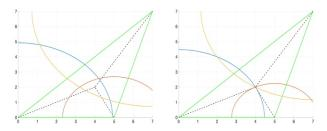
Figure 6: Iterative process for finding the Passive device position through circles intersection
