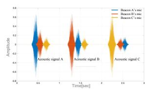
Figure 3: Multiple Active device signals recording with a single transmission per Active device
