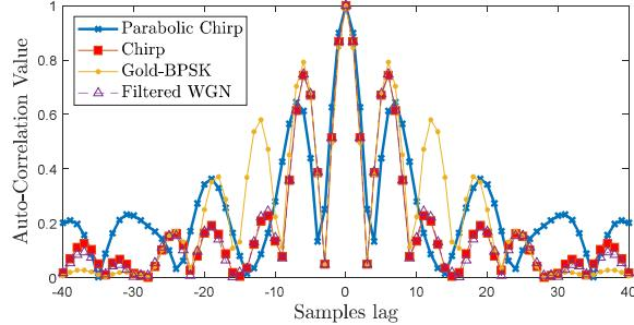
Figure 3 - Autocorrelation waveforms of the evaluated positioning signals
