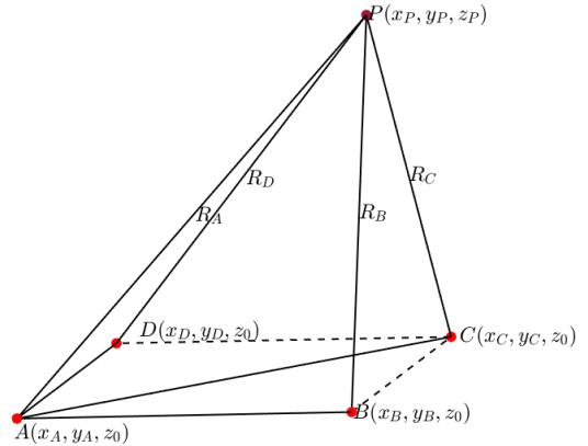
Figure 6 – Geometric layout of the system elements - beacons A, B, C, D and a mobile device P.
