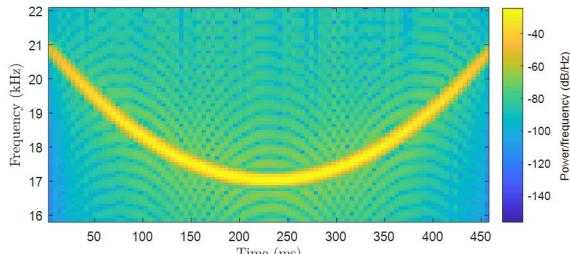
Figure 2 - Spectrogram of a parabolic chirp
