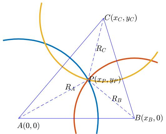
Figure 5 – Geometric layout of the system elements - beacons A, B, C and a mobile device P at the intersection point of the three circles.
