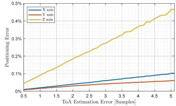
Figure 11 – Positioning error percentage per each axis as a function of ToA estimation error.
