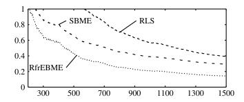
**Fig. 1.** MSE/ $||x||^2$  as a function of the number of observations for RLS, SBME and RfrEBME. The input is a square wave with a period of  $2\pi$ . The filter is a 19th order FIR whose coefficients are proportional to the eigendirection having minimal variance. The effective dimension and modified effective dimension rise steadily with n and converge to 9.3 and 6.9, respectively.
