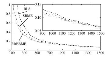
**Fig. 2.** MSE/ $\|x\|^2$  as a function of the number of observations for RLS, SBME and RfrEBME. The input is a randomly generated IID signal. The filter is a 10th order Butterworth low-pass with a cut-off frequency of  $\pi/2$ . The SNR is -20 dB. The average effective dimension and average modified effective dimension converge to 9.5 and 7.5, respectively. The inlaid graph displays the same results in a different scale.
