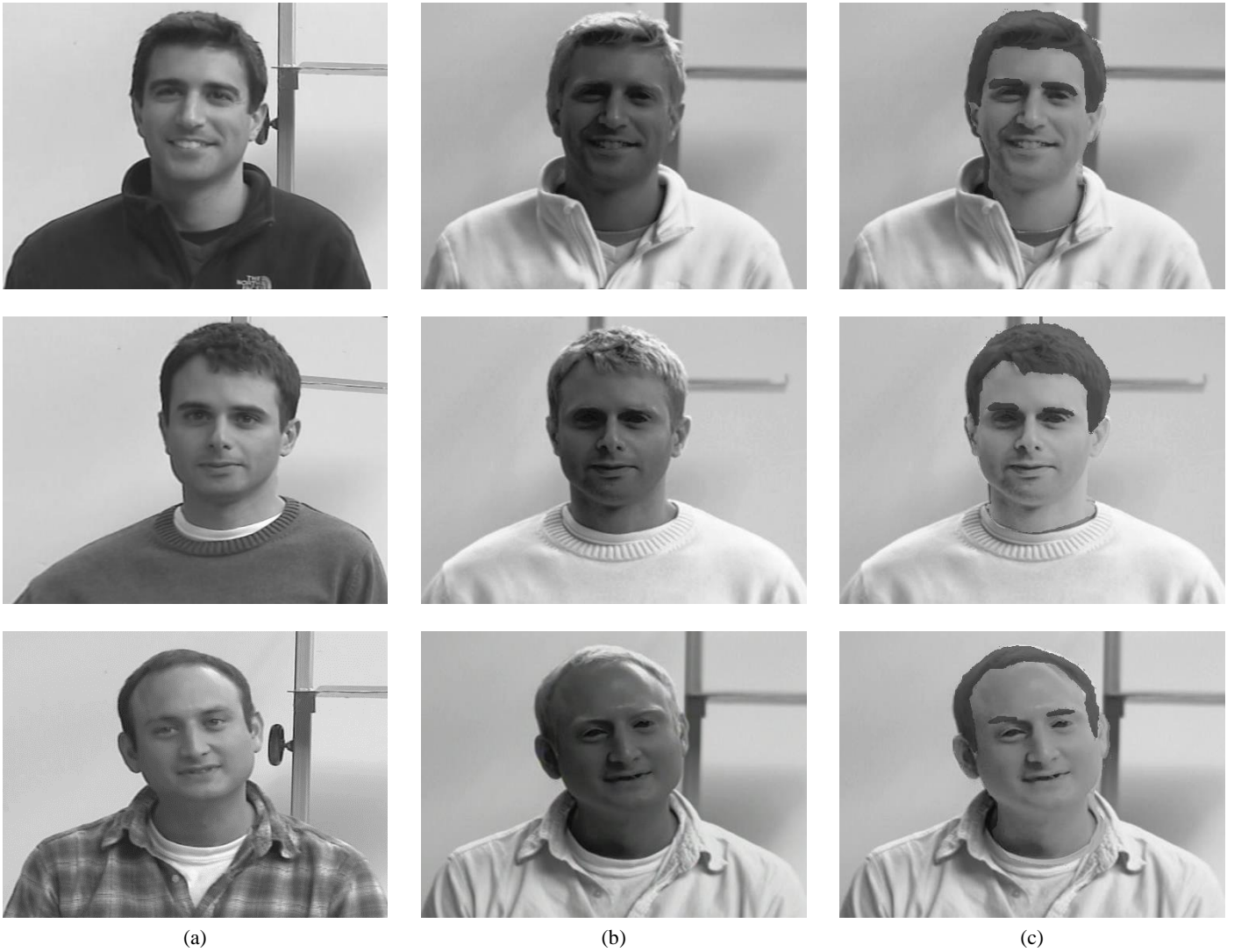
Fig. 4. Subject faces acquired outdoor at daytime in (a) visible band, (b) SWIR band, and (c) SWIR band after tone mapping using the proposed technique.
