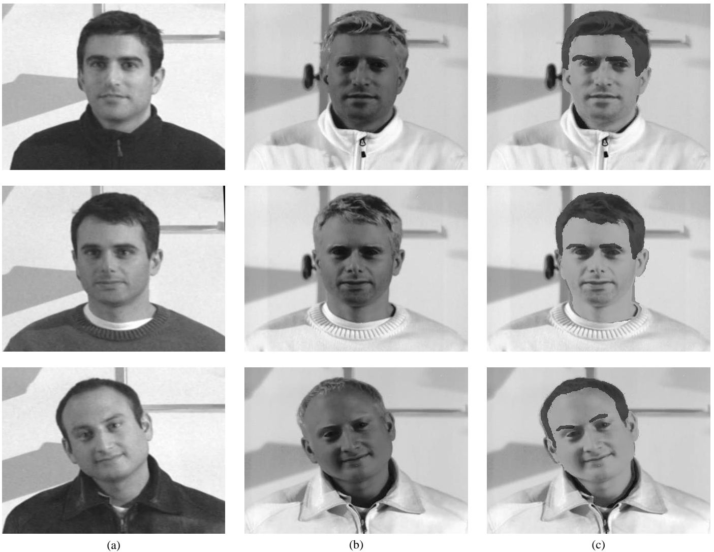
Fig. 5. Subject faces acquired outdoor at nighttime with street light illumination in (a) visible band, (b) SWIR band, and (c) SWIR band after tone mapping using the proposed technique.
